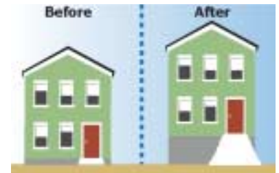
Figure 1-2: Elevation of structure above floodplain
